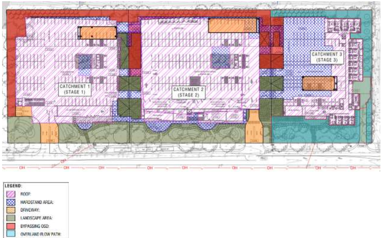
Figure 5: Internal Catchment plans and corresponding OSD tanks
